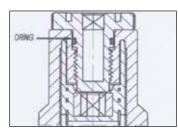
Place the O-ring cap of the perforator part and fasten it until it gets locked.
